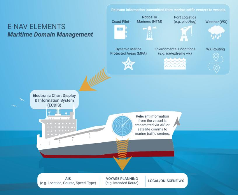
Using e-NAV technologies, it is possible to use a vessel's AIS to evaluate the vessel's location and destination, identify relevant data and information and transmit that information to the vessel's Electronic Charting Display and Information System (ECDIS) in real time. While this technology and means of disseminating relevant information exists, its implementation has been limited.
