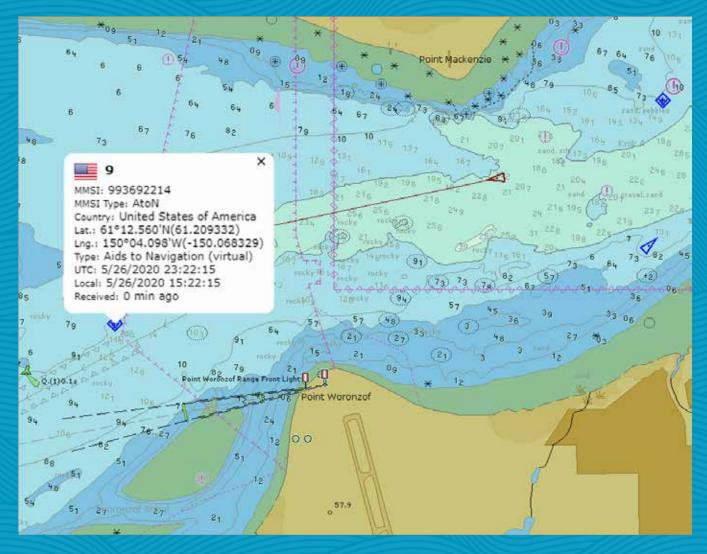
Location of virtual buoy transmitted via AIS.
